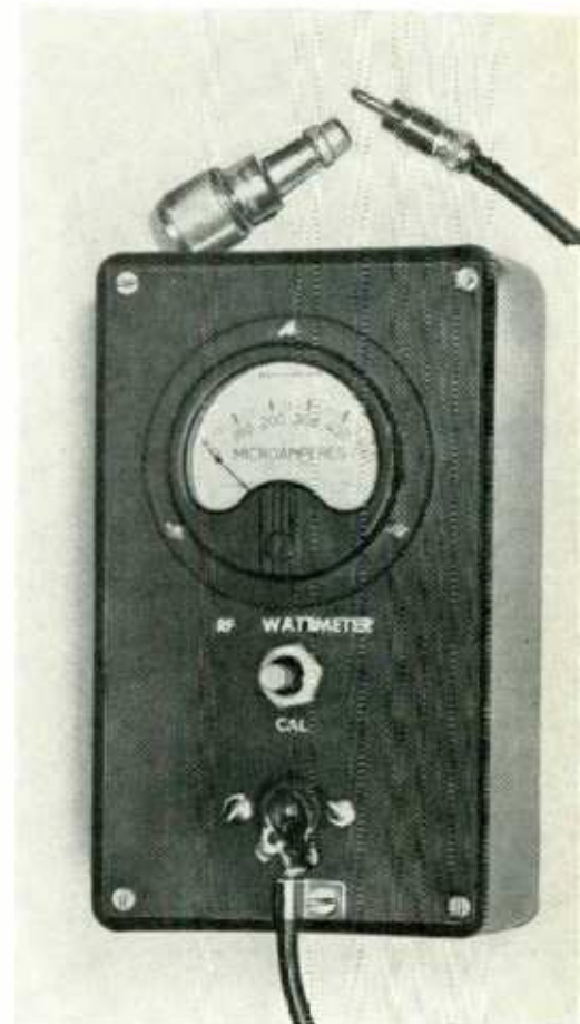
The wattmeter. Scale should be calibrated in watts. At top, cable ends in phono plug; adapter, top left, fits screw type coax connector. Other end of coax is soldered directly to lamp socket terminals, visible above clamp at bottom of case.
