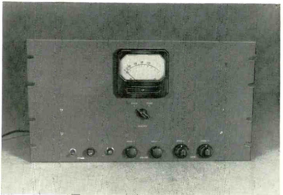
Finished product. Though shown here with oversize rack-mount panel, amplifier could be built into other equipment or housed in cabinet. VU meter and selector are not essential part of circuit.
